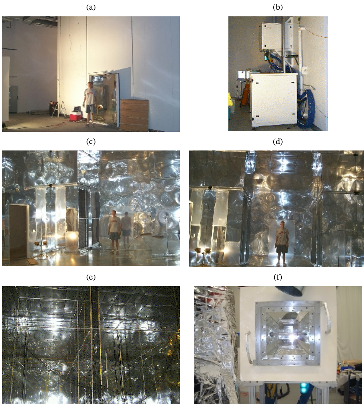
Figure 3. Photographs of environmental chamber enclosure and light source. (a) Outside the enclosure showing the access door. (b) Behind the enclosure showing the controls for the light. (c,d) Inside the enclosure showing the light and the air handler prior to the installation of the light and reflective material on the floor (light above the person's head in picture "d"). (e) Inside the enclosure showing the framework and netting that will hold the Teflon bag reactors in place. (f) Picture of lamp as taken at factory during testing.
