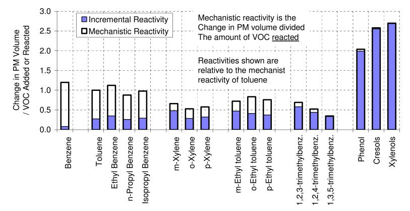
Calculated for the conditions of a standard UCR surrogate  $-NO_x$  chamber experiment using the SAPRC-11 aromatics SOA mechanism.
