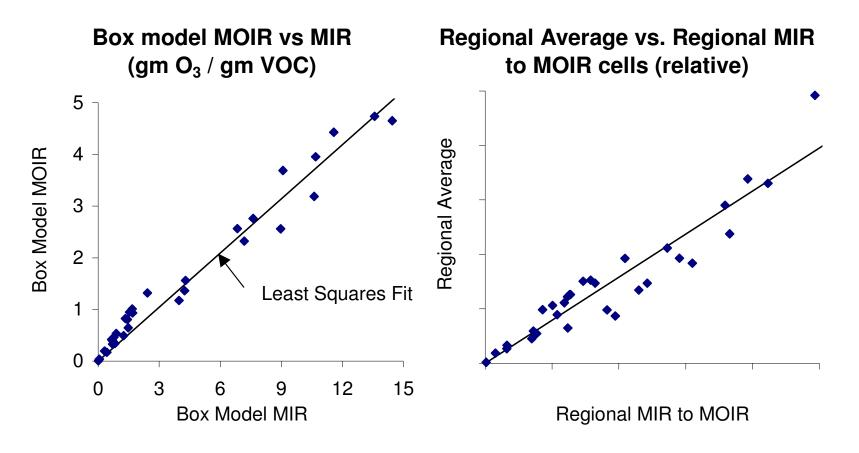
Box and regional model calculations used the SAPRC-99 Mechanism
