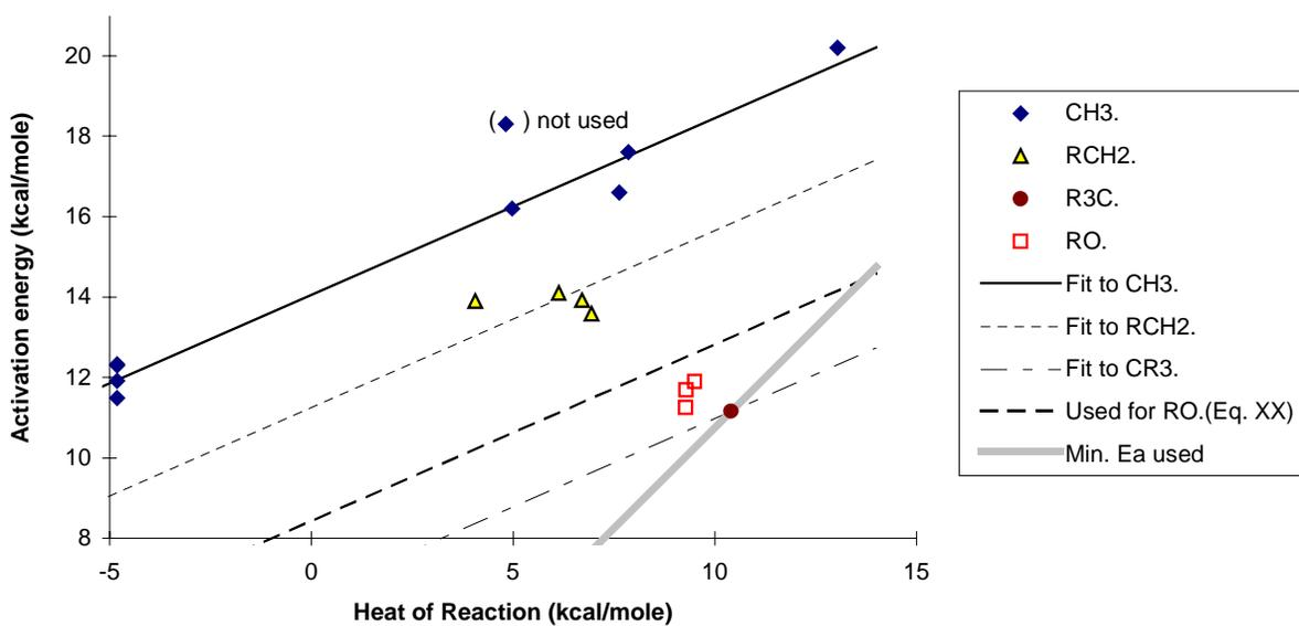
Figure 8. Plots of estimated or measured activation energies vs. heats of reaction for various alkoxy radical decompositions.
